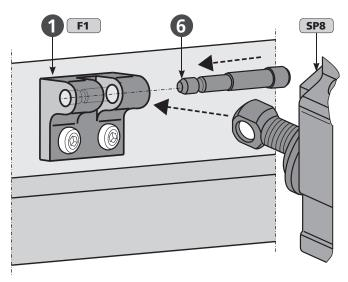
■ Optionally adjust the pressure ball • - of the casement bracket F1 • - with grub screw • and the spring •.
