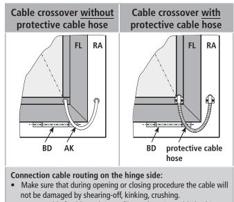
Protect cable feedthrough in profile e.g. by using cable bushings, cable transitions.
