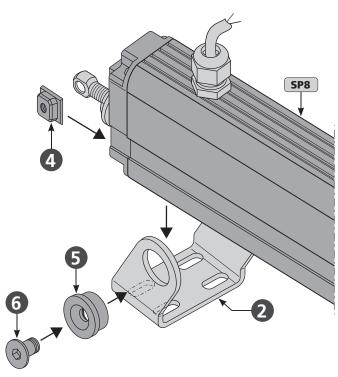
■ Tighten the clamping piece **⑤** with cylinder head screws **⑥** (torque 2,0 to 2,5 Nm).
