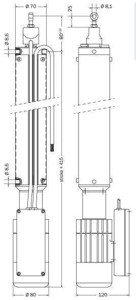
The compact drive design is fit for any type of linear movement. Connected to a high performance gear motor the principle of the trapezoidal thread spindle is applied for high shearing forces and speeds. All building components have anti-corrosion surface layers. The motor can be operated in parallel. The simultaneous control for the "Open" and "Close" direction causes a faulty drive.
