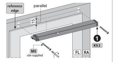
■ Screw th casement bracket **F95 ②** onto the casement - with on-site screws (**M5**).
