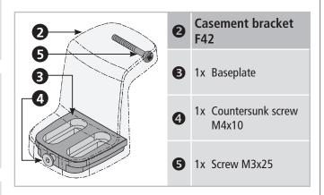
Note If necessary, use washers. These are depending on the type of screws used.
