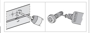
Note Screws - for mounting on the window - are to be provided by the customer!
