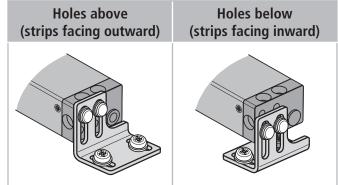
■ Tighten the KS 2 drive **⑤** with self-tappinge screws M5 **④** and washers **⑤** (max. 4 Nm).
