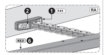
■ Route the connection cable on the transom. Cable must be protected against damage (shearing-off, kinking, splitting).
