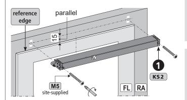
■ Screw the baseplate ③ from the casement bracket F42 ② onto the casement - with on-site screws (M5).
