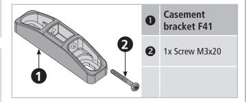
■ Mount the casement bracket **F41 ①** - with on-site screws (**M5**) - on the window casement.
