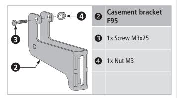
**NOTE** If necessary, use washers. These are depending on the type of screws used.
