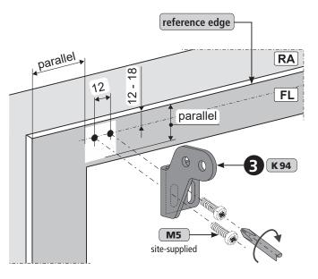
■ Secure the **KS 2** drive **⑤** with self-tapping screws **M5 ④** and washers **⑤** (max. 4 Nm).
