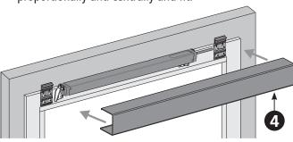
NOTE Ensure the correct positioning of the cover profile **4** (short side facing upwards).
