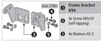
NOTE If necessary, use washers. These are depending on the type of screws used.
