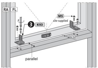
Note There are different mounting options for the frame bracket **K93 3**.
