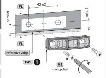
Note If necessary, use washers. These are depending on the type of screws used.
