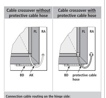
Make sure that during opening or closing procedure the cable will
