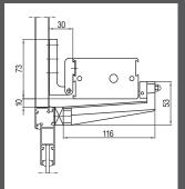
On the frame with the bottom hinged window brackets part No. 40625V and pivoting brackets part No. 40560T
