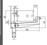
On the frame with the sliding fixing brackets included and the bottom hinged window bracket part No. 40625V
