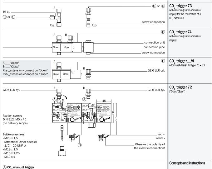
Opens by pressing the manual lever the CO<sub>2</sub>-bottle under it.
