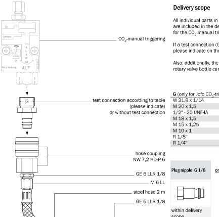
All individual parts in the drawing are included in the delivery scope, except for the CO<sub>2</sub> manual trigger.
