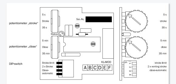
The comfort venting module KL-MOD is an expansion module for our smoke and heat ventilation control units (2A-1-1, 5A-1-1, 10A-4-1, 20A-4-1, 15A-1-1 24 V/36 V, 30A(20A)-2-1 24 V/36 V, 60A(40A)-4-1 24 V/36 V, 75A(50A)-5-1 24 V/36 V and the modular technic MC and MC60 in 24 V/36 V). If the module is plugged additional ventilation functions can be used.
