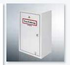
The smoke and heat ventilation control unit acts as a control unit for 24 V DC motor openers in max. one ventilation and one smoke and heat ventilation triggering group. The control function of the unit provides emergency power for max. 72 hours in the event of a power failure. The ventilation function is controlled via a double rocker switch and optionally, via a wind-rain detector.
