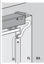
Drill hole in glazing bead (cable bushing protects against damage to cable).
