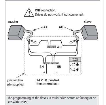
WH is used for communication, with synchronized multi-drive
