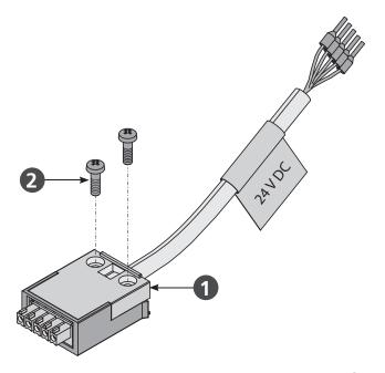
Note Locking hooks - at the housing cover ① - prevent withdrawal of the plug under tensile load.
