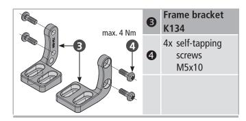
■ Fasten frame bracket **K134 ③** with screws (**M5**).
