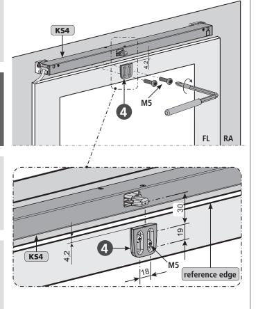
■ Slide casement bracket **F42 3** on the baseplate **4** and secure with screw **5**.
