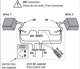
**WH** is used for communication, with synchronized multi-drive operation.
