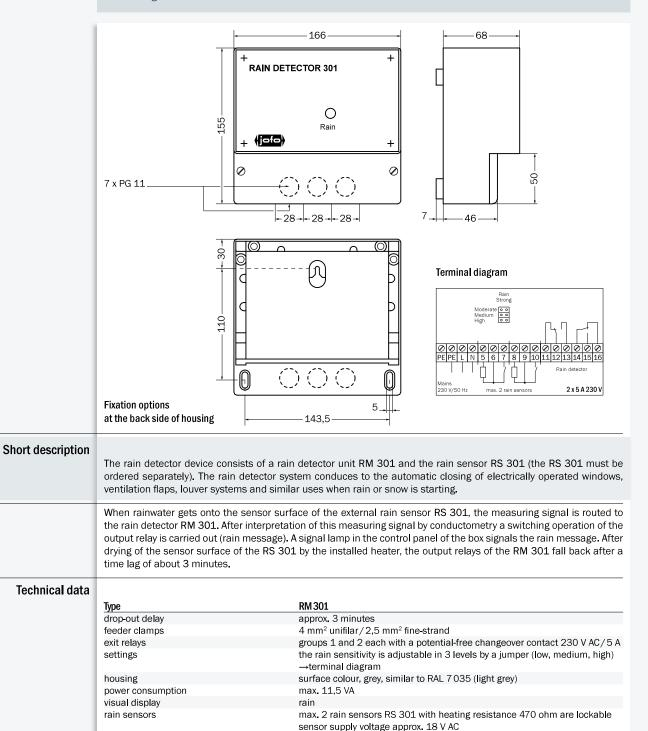
temperature class 3, as in VdS 2581 (-5 °C up to +40 °C)
