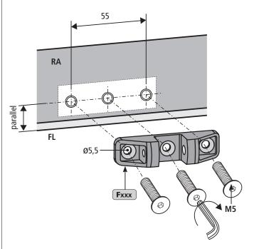
Secure fasteners against loosening; i. e. by applying removable thread-locking compound such as "Loctite".
