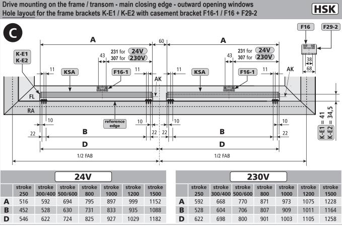
Drive mounting on the frame - main closing edge - outward opening windows Hole layout for frame brackets K-87 with casement bracket F16 / F33
