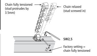
Always note the force-path diagram (see chapter **"Data sheet KSA S12"**) and rigidity of the chain, depending on the installed position!
