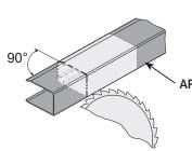
■ Check the swivel area of the drive and if necessary cut out the cover profile **AP** in the area of the brackets.
