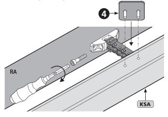
Route cable on the frame or mullion/transom. The drive and its connection cable are swivelling. As a consequence, foresee cable routing with a loop. Cable must be protected against damage (shearing-off, kinking, splitting).
