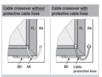
Connection cable routing on the hinge side:
