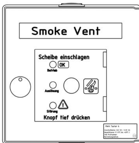
Smoke and heat vent switch 6
