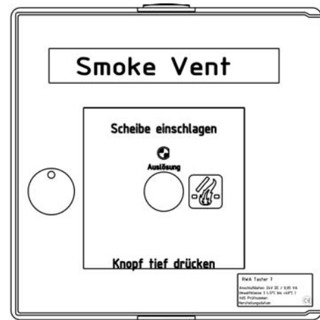
Smoke and heat vent switch 7
