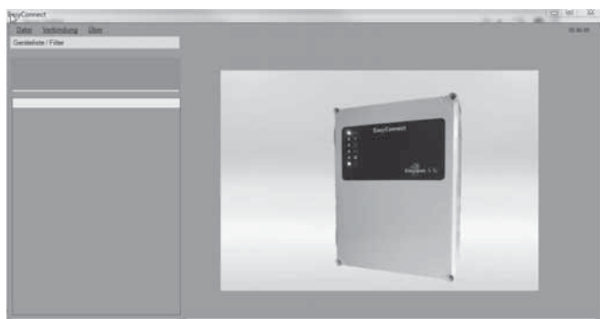
Fig.: EasyConnect configuration software start screen without the service port connecting cable connected.
