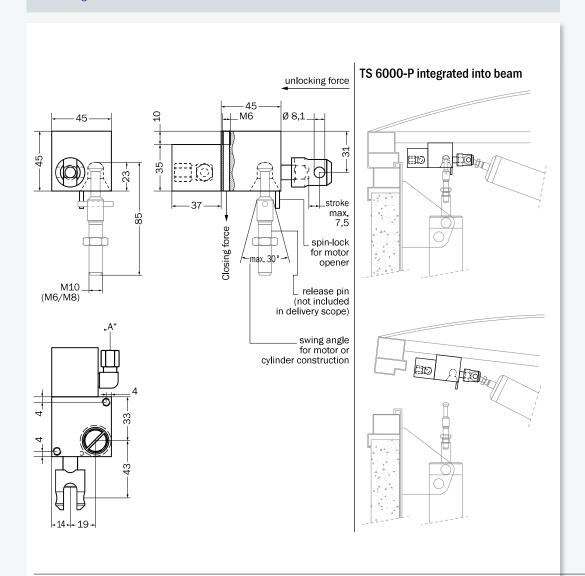
The traverse lock TS 6000-P is implemented for the smoke and heat ventilation control. As soon as pressure is exercised onto the clevis, the release pin is automatically released by the traverse lock. By the pressurization of the connection "A" the traverse lock is also released (for the monitoring of the smoke and heat ventilation control unit).
