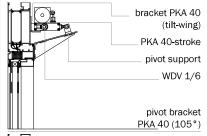
The pneumatic chain drive PKA 40 is fit both for the opening of the tiltwings and swing-wings. It distinguishes itself by its level position before the frame while it does not protrude into the room.
